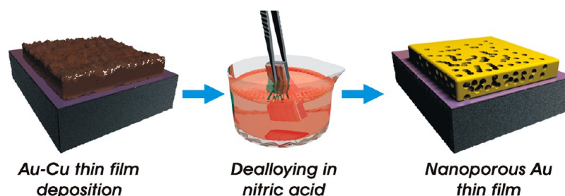
Figure 1. Scheme of the two-step fabrication process of nanoporous gold thin films based on the deposition of Au–Cu alloy followed by wet etching in nitric acid.
